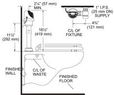
When installing the G2° Hardwire in a handicap stall: Per the ADA Guidelines (section 604.9.4) it is recommended that the grab bars be split or shifted to the wide side of the stall.
