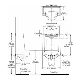
NOTE: ADA urinal rim height requirements allow all heights 17<sup>\*</sup> and below. Sloan strongly recommends roughing in the drain to achieve a 16<sup>+/\*</sup> rim height or less to ensure compliance.
