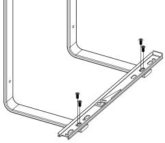
3) Once both inner slides member are attached to both sides you are now ready to attach the brackets to a underside of your shelf using the provided (4) wood screws.
