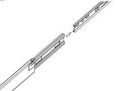
2) Lay both brackets on one side and attach the inner slide member to the brackets using the provided machine screws.
