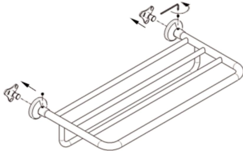
② ALIGN MOUNTING BRACKETS AND MARK LOCATION
